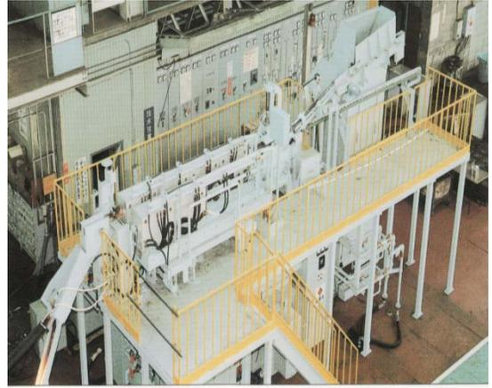
**750KW 3000Hz modular type billet heater**
